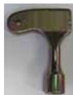
Figure 4: Auto Slim Landing Doors Emergency Opening
